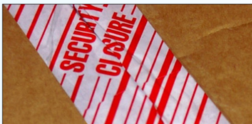
1248 slit and resealed with a clear packaging tape. Printed diagonal lines clearly indicate tampering.
